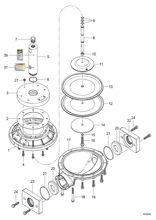
Fig. 6. i200 (DTE) parts exploded view, aluminum model shown
