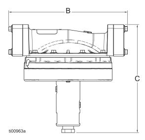
FIG. 7. Dimension Diagram for i100 (DTC)
