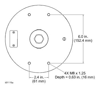
Fig. 2: Mounting thread dimensions
