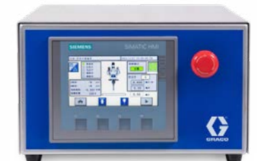
Integrated PLC Controller
