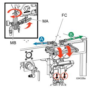
6. Open the motor air shutoff valve (MA).
