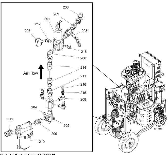
Fig. 8: Air Control Assembly 26C417
