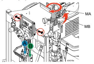
**XP-h Systems only:** Set pump valve on. Then turn down the pressure control knob.
