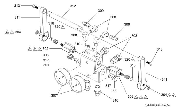
Apply anaerobic pipe sealant to all non-swiveling pipe threads.
