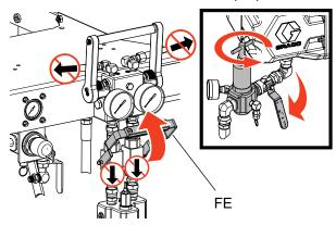
5. Open the solvent pump air valve (DA). Slowly turn the solvent pump air regulator (DB) clockwise to increase air pressure.
