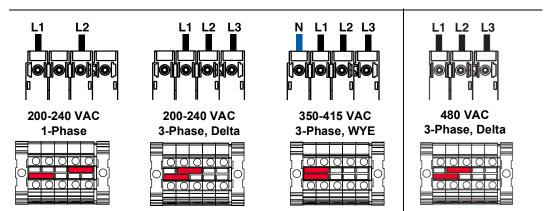
Fig. 7: Terminal Jumpers and Positions
