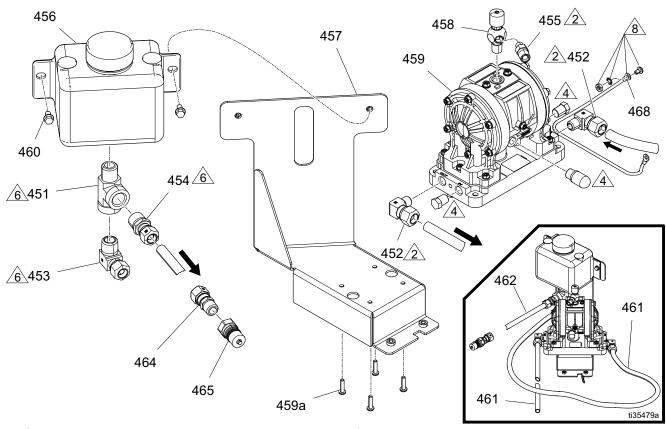
Apply thread sealant to all non-swiveling pipe threads.
