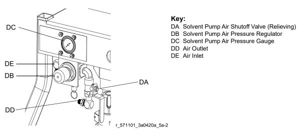
Fig. 6: Solvent Flush Pump Kit Air Controls
