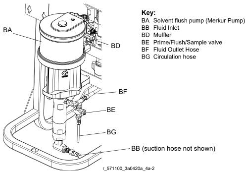
Fig. 5: Solvent Flush Pump Kit Pump
