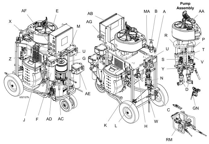
Fig. 1: XP70 Complete System (model 576107 shown)
