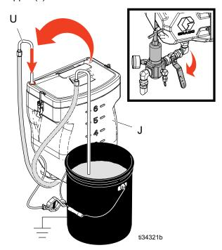
If using heaters, heat fluid throughout system before spraying. See Recirculate Prior to Spraying or Re-Prime After a Pump Runs Dry, page 34.
