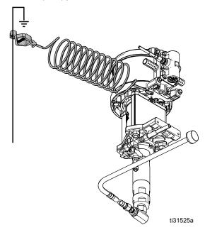
**Air and fluid hoses:** use only static dissipation type hoses with a maximum of 300 ft (91 m) combined hose length to ensure grounding continuity. Check electrical resistance of hoses regularly. If total resistance to ground exceeds 29 megohms, replace hose immediately.
