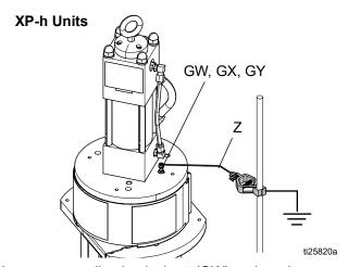
Loosen grounding lug locknut (GW) and washer (GX). Insert ground wire end (Z) into lug (GY) slot and tighten locknut securely. Connect ground clamp to a true earth ground.
