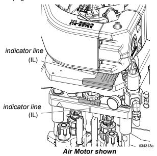
Verify that the motor position is adjusted correctly for that mix ratio (refer to the image above). If not, follow the **Change Motor Position** procedure on page 26.
