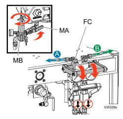
2. Lift to close the circulation handle (FC) when the pump is at the bottom of the stroke.
