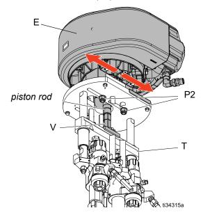
5. Grab the piston rod and slide the position of the motor (E) until the indicator lines are aligned with your ratio.
