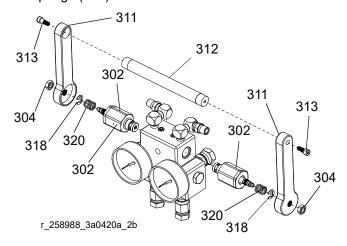
4. Unscrew both over pressure relief valves (302) from the manifold.
