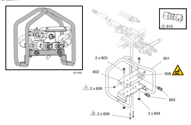
Apply thread sealant to all non-swiveling pipe threads.
