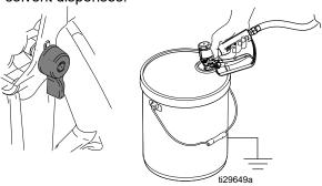
8. Close the solvent pump air valve (DA). Trigger the gun to relieve pressure. Close the solvent flush valve (FD) after relieving the pressure.
