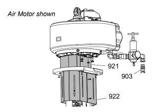
5. Use a wrench to hold the tie rod (902) flats to keep the rods from turning. Unscrew the nuts (908) and washers (907) from the tie rods.
