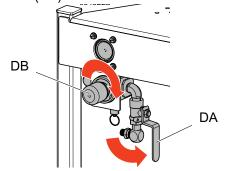
Open the solvent flush valve (FD) on the mix manifold.
