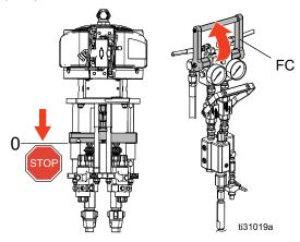
Close the motor air valve (MA) and turn the air regulator (MB) counterclockwise. Lower to open the circulation handle (FC).
