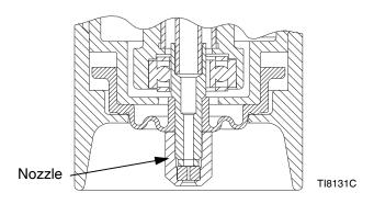
Fig. 7: Deflector and Nozzle Detail
