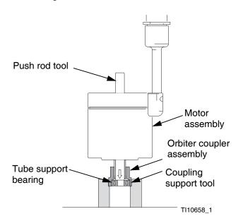
Fig. 2: Coupler Assembly Removal
