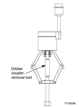
Fig. 3: Remove Orbiter Coupler
