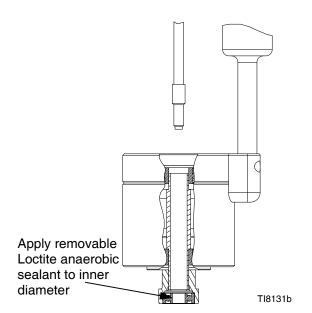
Fig. 6: Tube Assembly - End Detail
