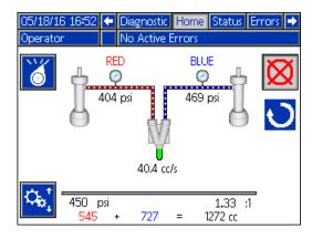
Fig. 32: Main Operator Mode Run Screen, Dispensing in Constant Pressure Mode.
