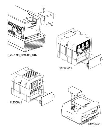
Fig. 17: Remove Access Cover
