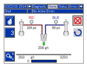
Fig. 41: System Circulating Automatically after a Shot Mode Dispense
