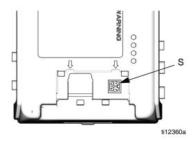
**Low Power Module Rotary Switch Location**
