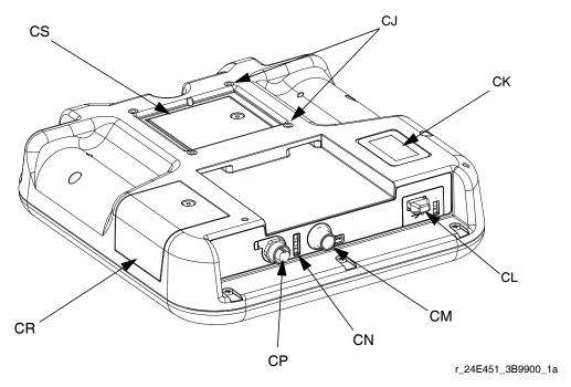
Fig. 6: ADM Component Identification - Rear
