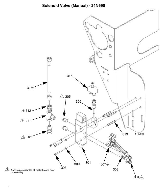
Fig. 30: HFR Semi and Fully Automatic Valve Kit
