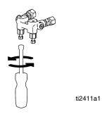
For models with an MD2 valve, connect whip hose to MD2 valve component A (Red) and component B (Blue) fluid inlets.
