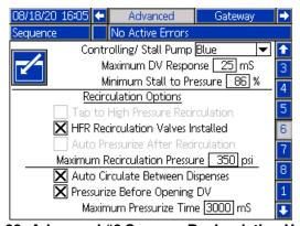
Fig. 28: Advanced #6 Screen - Recirculation Valves Installed Option
