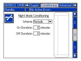
Night Mode is available for full recirculating systems (L-Head, S-Head, and S-Head w/ Prox valve options), and systems with semi-automatic recirculating kits installed (refer to **Appendix H- Circulation** on page 115 for recirculating kit details).
