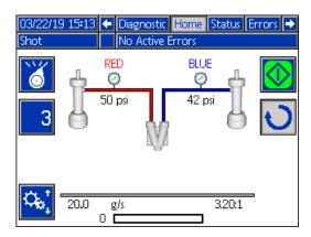
Fig. 38: Shot Mode with System in Circulation Configuration
