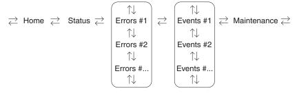
Fig. 25: Run Screens Navigation Diagram
