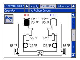
2. Press to display the setpoint and alarm values associated with that component.
