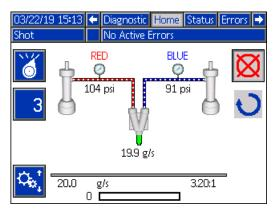
Fig. 39: Shot Mode with System Circulating Material
