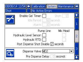
Post Dispense Shot Disable is a feature where the user can disable shot requests for zero to five seconds after the completion of a dispense. This feature is not applicable for P2/Fusion Dispense Valves. This feature can not be active if the Pre Dispense Delay feature is active.
