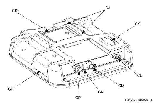
Fig. 20: ADM Component Identification - Rear
