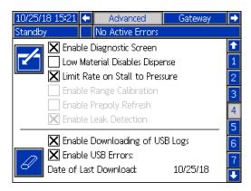
• Limit Rate on Stall to Pressure: Check this box to allow the HFR to increase to stalling pressure at a slower, more controlled rate.
