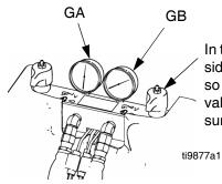
In this example, B (Blue) side pressure is higher, so use the B (Blue) side valve to balance pressures.
