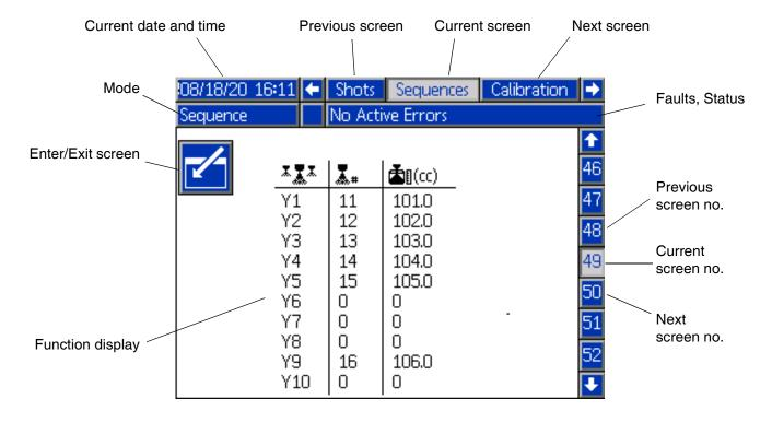
Fig. 7: Main Display Components
