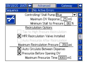
Fig. 44: Pressurize Before Opening DV Feature ON
