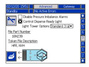
If the data on the token is not recognizable or the token is blank, the screen will display a message reading "Token Data NOT Recognized." If another token needs read, insert the next token and drigger
