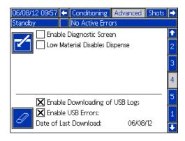
The first option is a checkbox that enables or disables the downloading of the Error Event and Shot Data log files. The Shot Data log runs during all circulation, shots, and operator modes.
