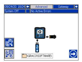
Insert the USB stick with the updated software file into the bottom of the ADM, and insert the black programming token into the right side of the ADM. The token does NOT need to be blanked. The process will blank and write the file from the USB stick to the token.
