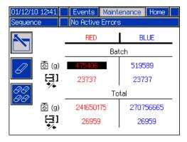
**NOTE:** In a circulation system, the pumpline must be stopped to erase counters.
