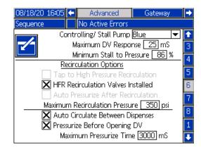
Fig. 36: Fully Automatic Circulation Feature ON
