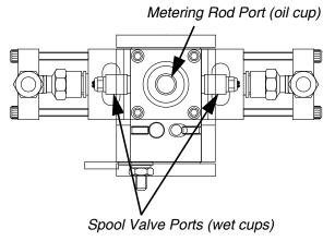
Fig. 8: Top View of Metering Valve with Top Section Removed
