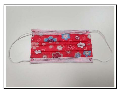
Dimension of the test specimen: 170 mm x 100 mm Size of the area tested: 49 cm<sup>2</sup> Flow rate during testing: 28,3 l/min Inner side of the mask to the aerosol challenge.
